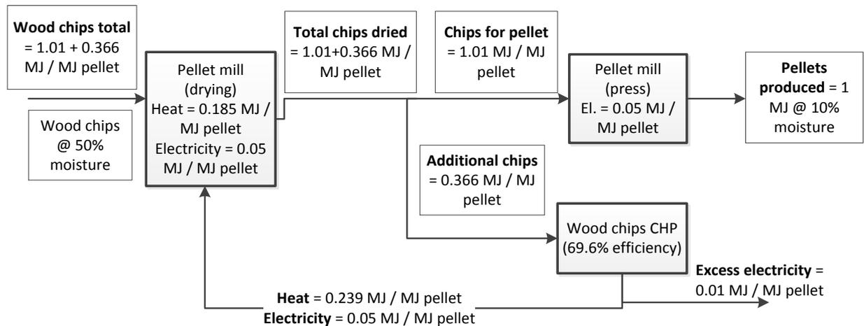
In the case of a CHP engine fuelled with wood chips it is not possible anymore to dimension the CHP on the power needs only, because the heat requirement would not be fulfilled. Therefore, the CHP is dimensioned over the heat demand and an excess electricity is exported to the grid.
