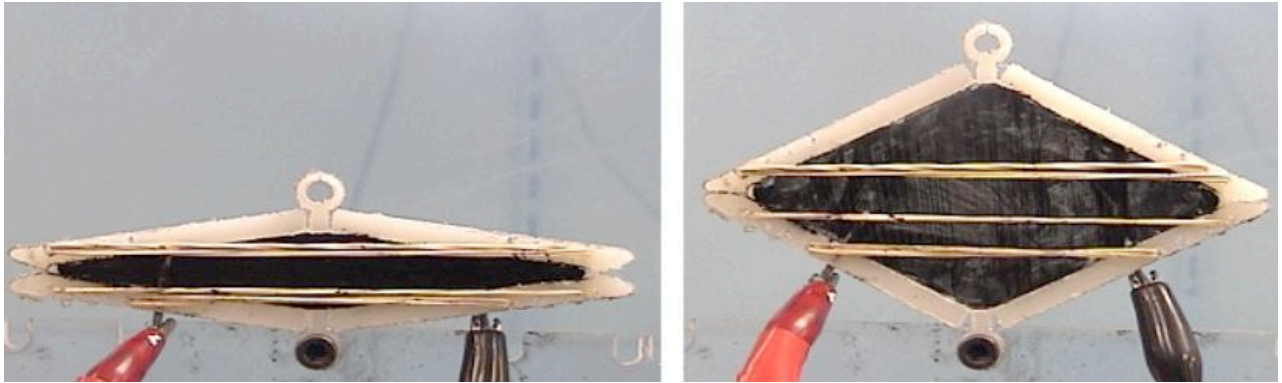
Figure 19: Experimental dielectric elastomer actuator showing 200 percent strain.
