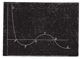
Hence the relation between pressure and volume may be represented by the curve  $A \ B \ C \ D \ E \ F \ G$ , where the horizontal ordinate represents the volume, and the vertical ordinate represents the pressure.
