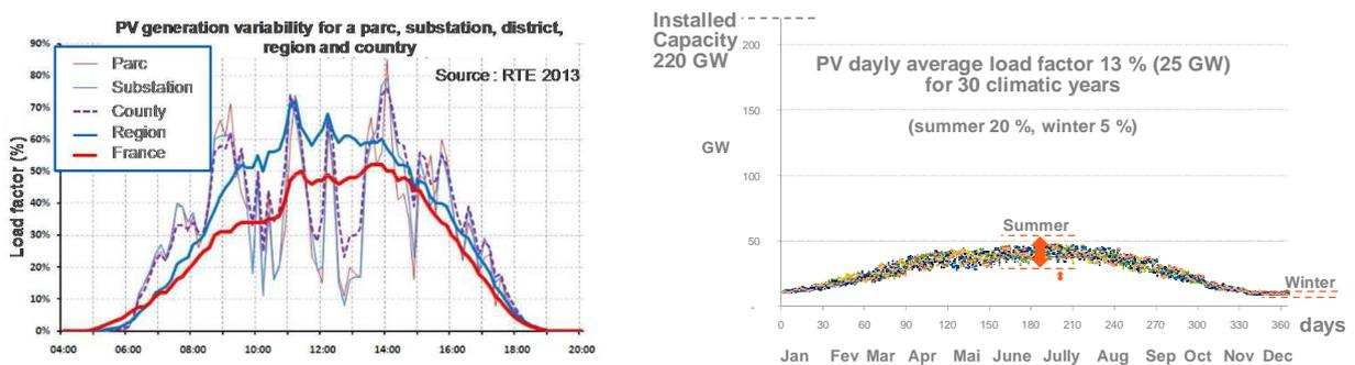
PV generation differs from wind in terms of level of its grid connection. A significant proportion of installations, including small roof-top arrays, are connected at low voltage with low observability and little or no controllability.
