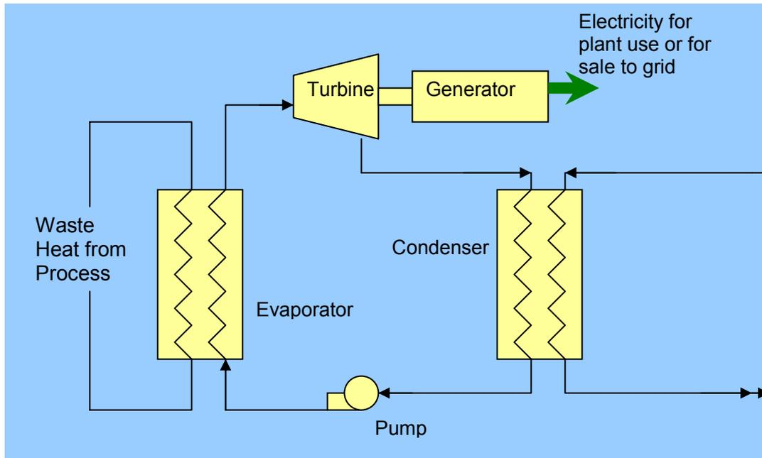
**Figure 18 - Waste Heat Recovery with Rankine Cycle -**
