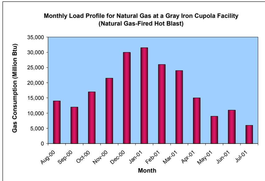
**Figure 26 – Example of Monthly Load Profile for Natural Gas at a - Casting Facility Located in the Midwest -**
