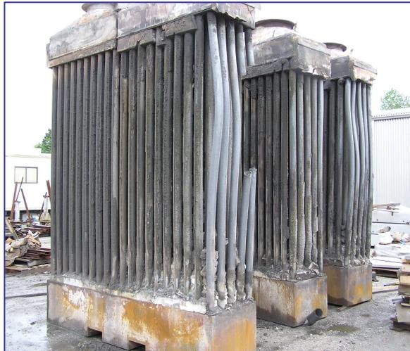
**Figure 3 - Abandoned Recuperator from an Aluminum Melting Furnace** (Source: ORNL)
