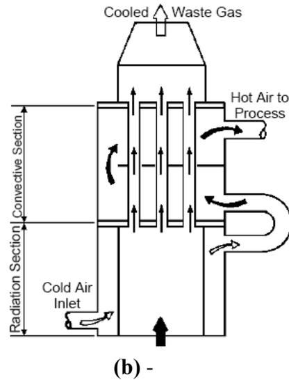
**Figure 5 - (a) Convection Recuperator (Source: Allstom, 2007), - (b) Combined Radiation/Convection Recuperator (Source: PG&E)**
