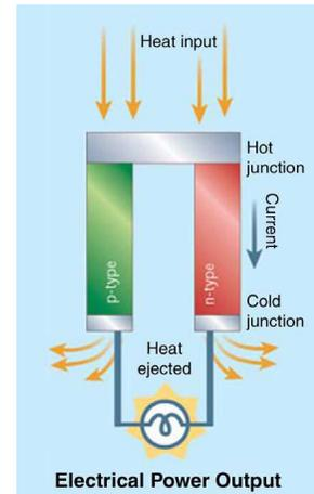
**Figure 20 - Thermoelectric - Generation Unit -**
