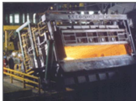
**Figure 25 - Gas-Fired Aluminum - Reverberatory Tilting Furnace -**
