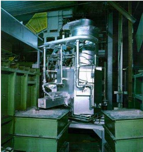
**Figure 12 - Stack Melter in a Die - Casting Facility -**
