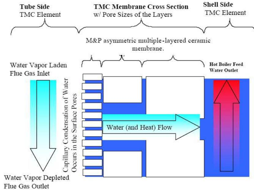
**Figure 15 - Transport Membrane Condenser** (Source: Liu, 2006)
