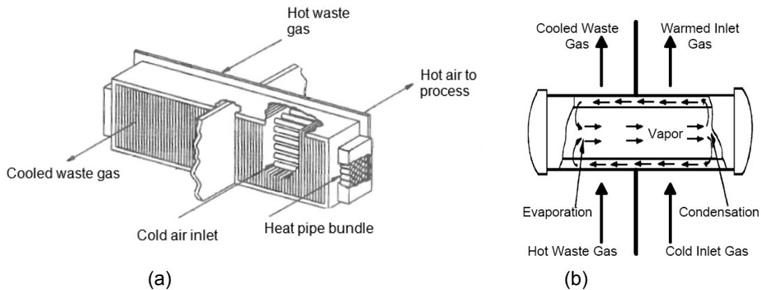
**Figure 9 - (a) Heat Pipe Heat Exchanger** (Source: Turner, 2006),
