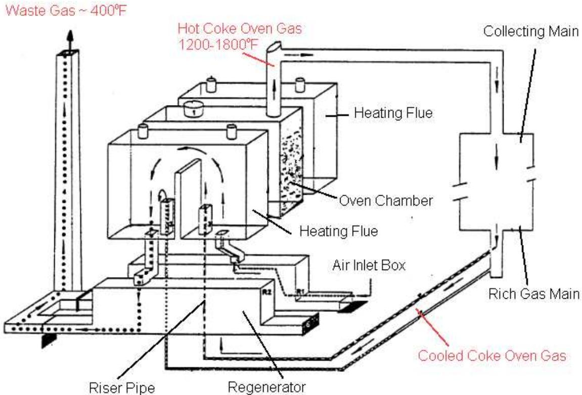
**Figure 22 - Coke Oven** (Source: IPCC, p. 113)
